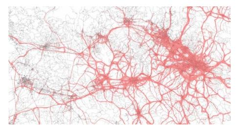
The GPS device captures the position ~ every 30 second with a 10 meter precision. Sample coverage is nearly 10% of actual Tuscan vehicle population. Since the data is very micro by nature, **spatial and temporal**
